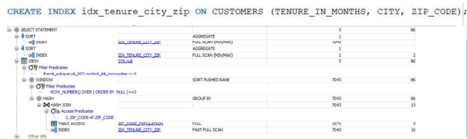
Fig. 15. Plan for Fastest-growing cities based on new customers with index
